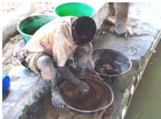
Fig. 3 – Amalgamation of gravity concentrates in Rwamagasa
