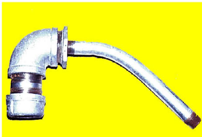
*Retorts can reduce drastically mercury emissions. Home-made retorts are not expensive. They can be made with water pipes and connections (devised by R. Hypolito)*
