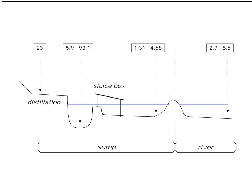
Figure 4- Schematic representation of mercury losses during gold extraction
