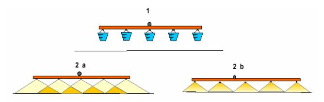
It is need to check the sprayer and calibrate it before work season. 1 Choose nozzles of equal discharge 2. Choose optimal boom height above plants that solution would cover the plants more equally: 2a - when spray patterns overlap, 2 b - when spray patterns do not overlap
