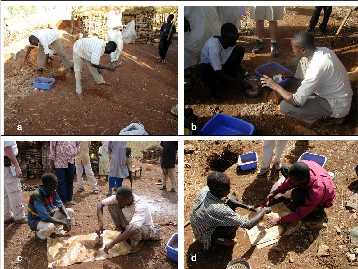
Illustration 26 - Soil sampling phases – (a) digging along line or point (b) sieving (c) division (d) collection in bottles.
