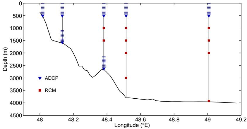
Figure 4: Instrumentation on the INATEX East Madagascar Current array, with the observed bottom topography.
