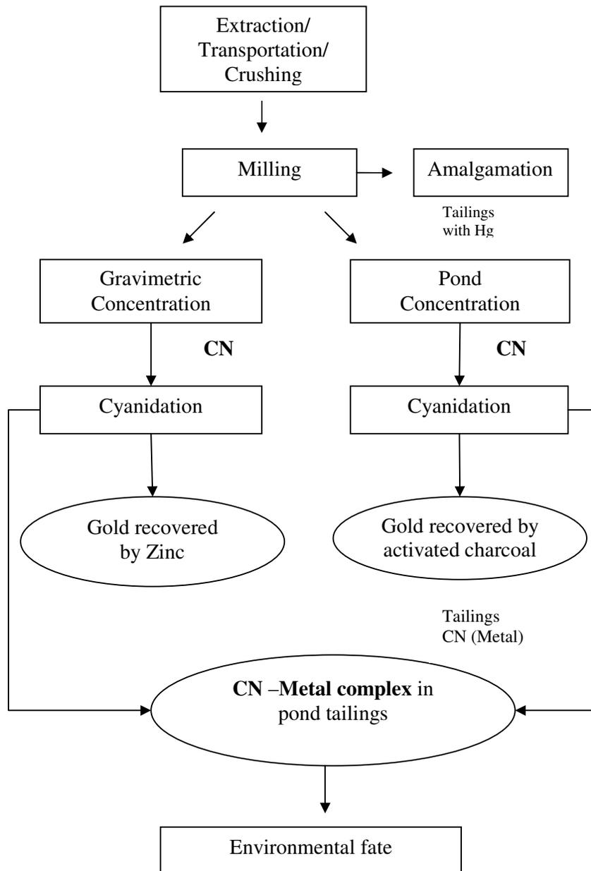
Fig 3. Simplified flowchart of common gold processing by Amalgamation and Cyanidation
