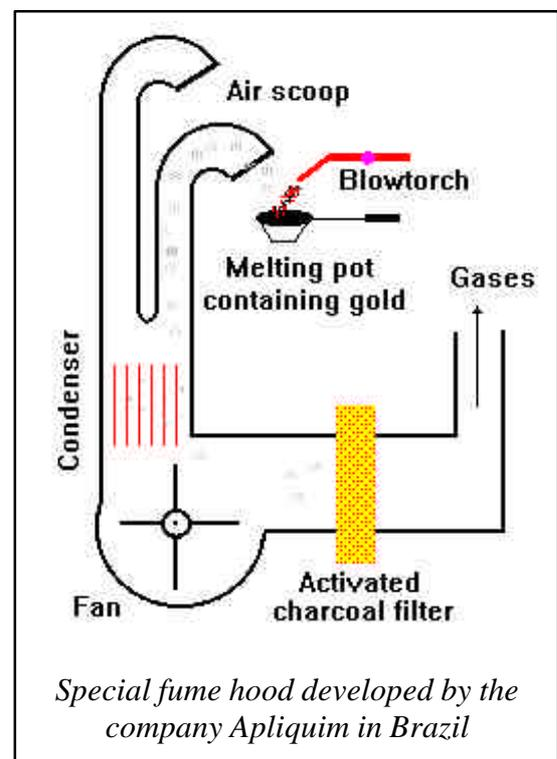
In 1989, a Brazilian company, Apliquim, developed a mercury condensing fume-hood consisting of a series of condensing plates coupled with iodide impregnated activated charcoal filters. This equipment reduces mercury emissions by more than 99.9%. Less than  $1 \mu\text{g}/\text{m}^3$  (WHO limit for public exposure) of mercury was detected in the exhausting gases of this fume hood.
