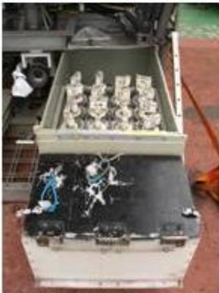
**Fig. 3:** Portside drawer with 16 pushcores and large lidded biobox in front
