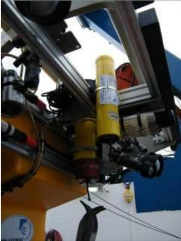
Figure 113. Sonardyne transponders mounted on light rack of the ROV, the smaller one served as a back-up.
