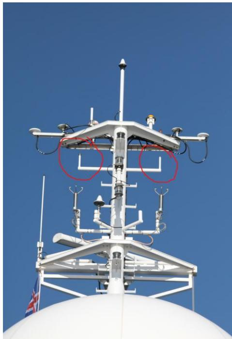
Figure 94. One possibility would be to use the two spare poles on the mast for science wind speed sensors. This would reduce shadowing by the vessel super structure and would offer additional readings to the wind sonic on the Met platform and Bridge DP system.
