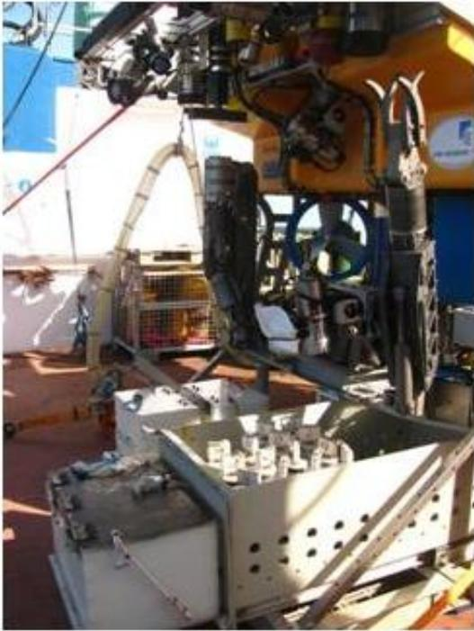
**Fig. 2a:** ROV KIEL 6000 with Configuration 1: port drawer with 16 pushcores and lidded biobox in front; starboard drawer with 2 lidded bioboxes.
