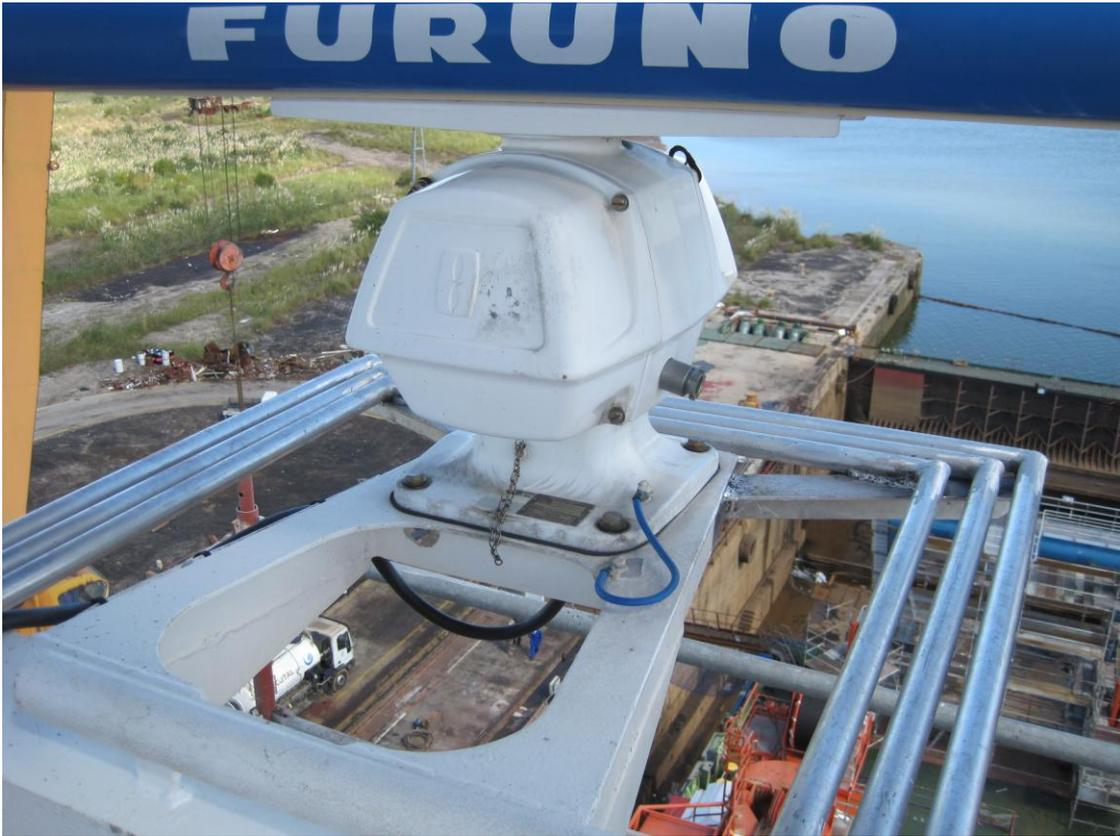
Figure 100. Access to the motor assembly is impossible with a man cage and access by an engineer on the mast is very difficult even with the new platform assembly.
