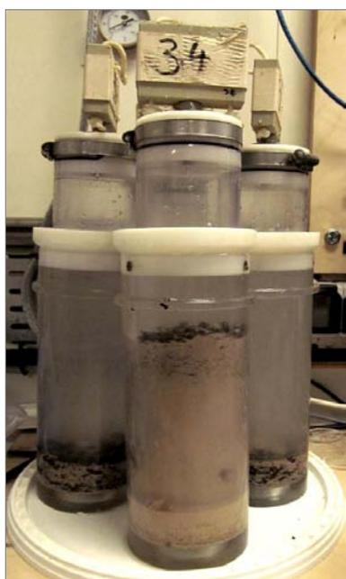
Figure 44. An example of a good, quantitative ROV push core (front) with two examples of poor cores, suitable only for use as qualitative samples, on either side.
