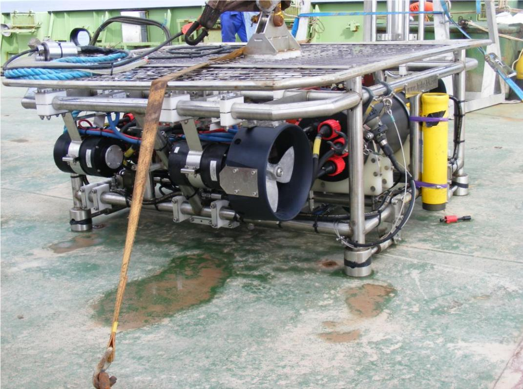
Figure 90. HYBIS showing the mounting of the USBL system.
