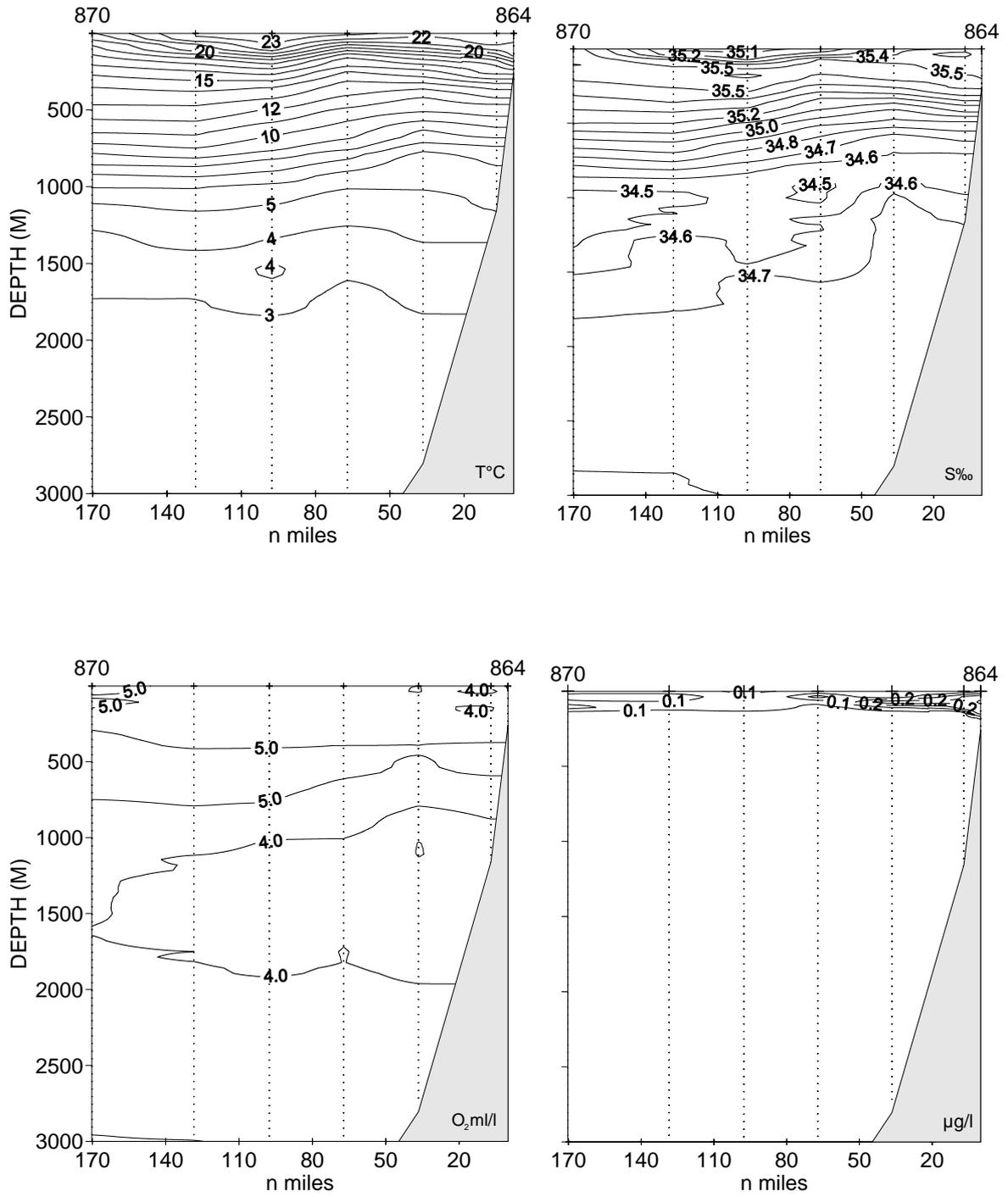
Fig. 3.3. Vertical sections of temperature, salinity, oxygen and fluorescence
