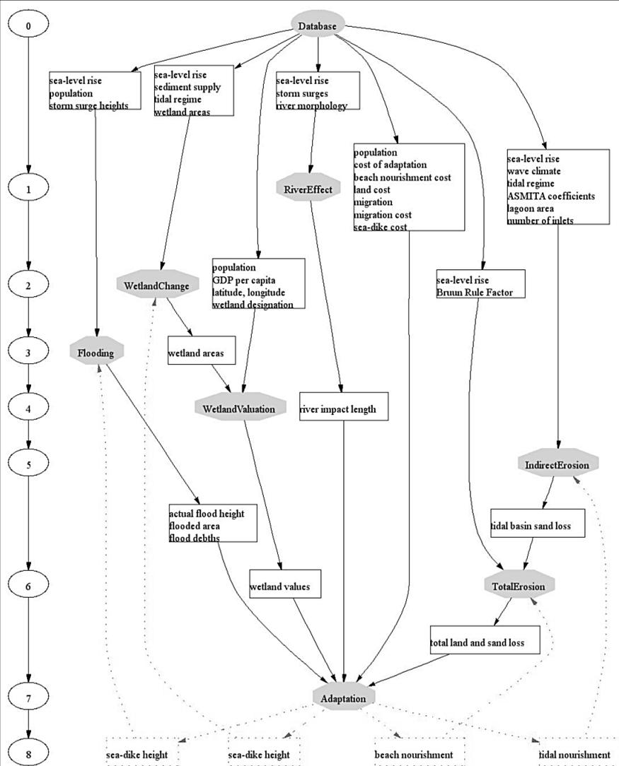
Figure 2 — Module linkages in the DIVA tool as of June 2003. This diagram is automatically generated by the DIVA documentation system. Ovals represent the modules, boxes represent data, the drawn through arrows represent the flow of data during one time step and the dotted arrows represent the data fed into the next time step.
