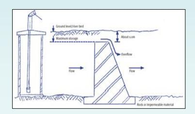
schematic drawing of subsurface dam
