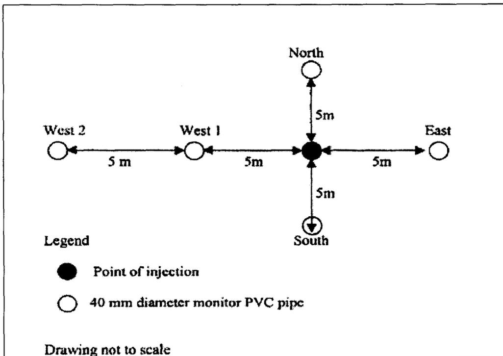
**Figure 2.1: Plan view of Small Scale tracing experiment**
