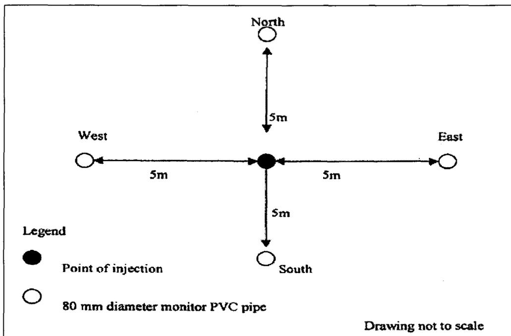
**Figure 2.2: Plan view of Large Scale Bromide tracing experiment**
