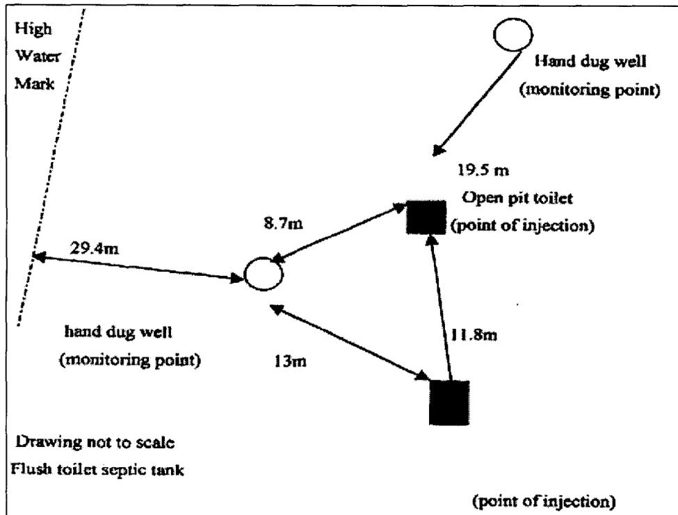
**Figure 2.4 Plan View of Large Scale dye tracing SITE 2**
