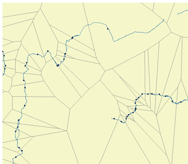
Figure 5.11: Rivers segmented on the basis of location in Thiessen polygons of water quality measurement stations. Attributes of water quality measurement stations are assigned to corresponding river segments.
