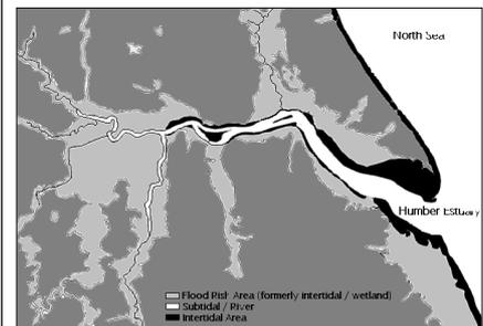
**Figure 2. The modern Humber Estuary.** The black area indicates present-day intertidal area, the light grey area represents original intertidal area (ca. 3000-300 years ago), prior to any reclamation; this area is currently below the level of high water spring tides and is protected by coastal defences (modified from Andrews *et al.* 2000).
