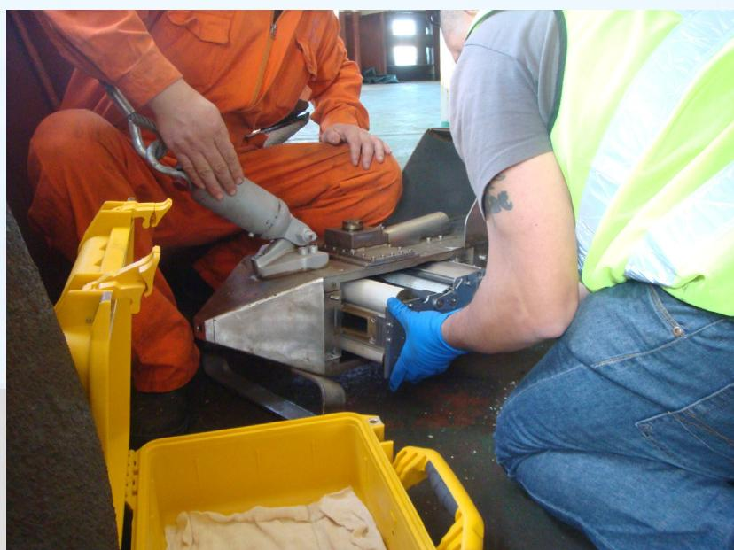
*Loading an internal plankton sampling mechanism into the CPR body.*
